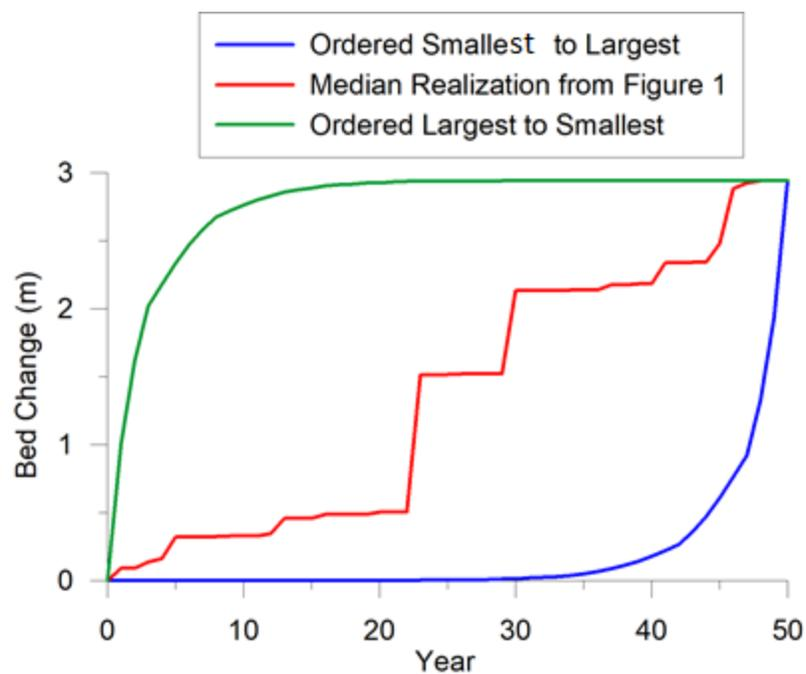
**Figure 2.** Median bed change time series from previous plot (red), reordered from max-to-min bed change (green) and min-to-max bed change (blue) to demonstrate the morphological impact of event timing on flood risks. If the larger events occur earlier project benefits are likely negatively impacted or project O&M expenses may be significantly increased.
