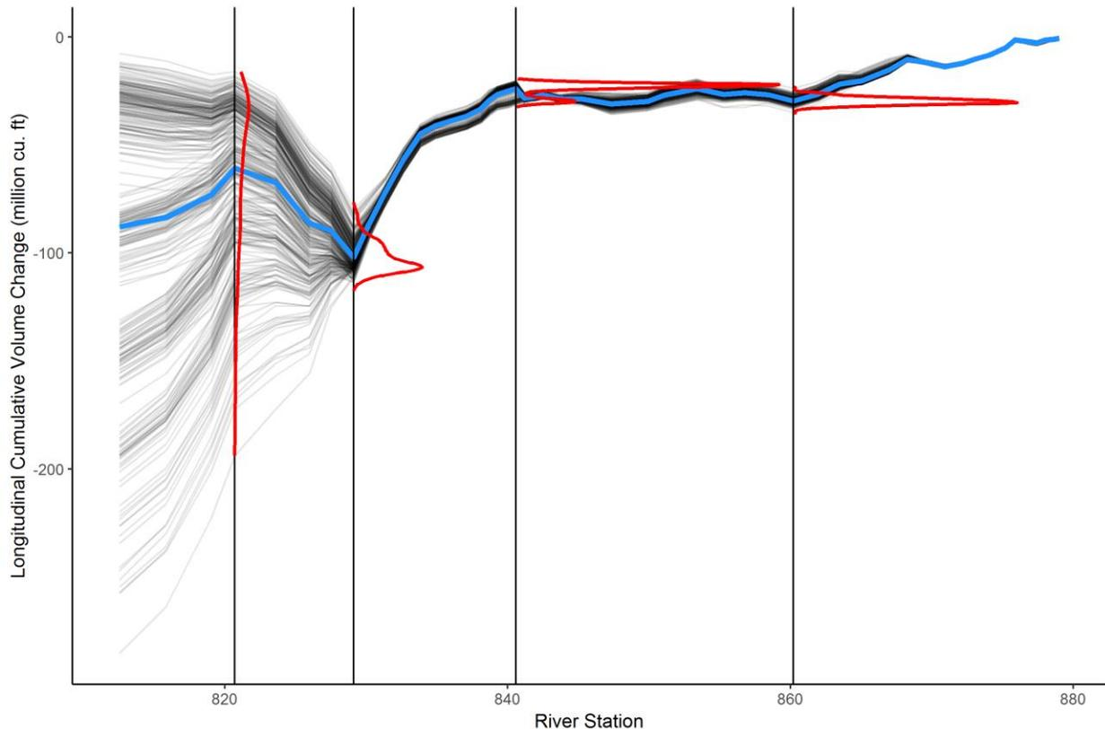
**Figure 4.** Longitudinal cumulative volume profile for 300, 50-year, mobile-bed, sediment-transport simulations with different hydrologic realizations from HEC-WAT. The blue line is the mean and the red lines are distributions at different locations.
