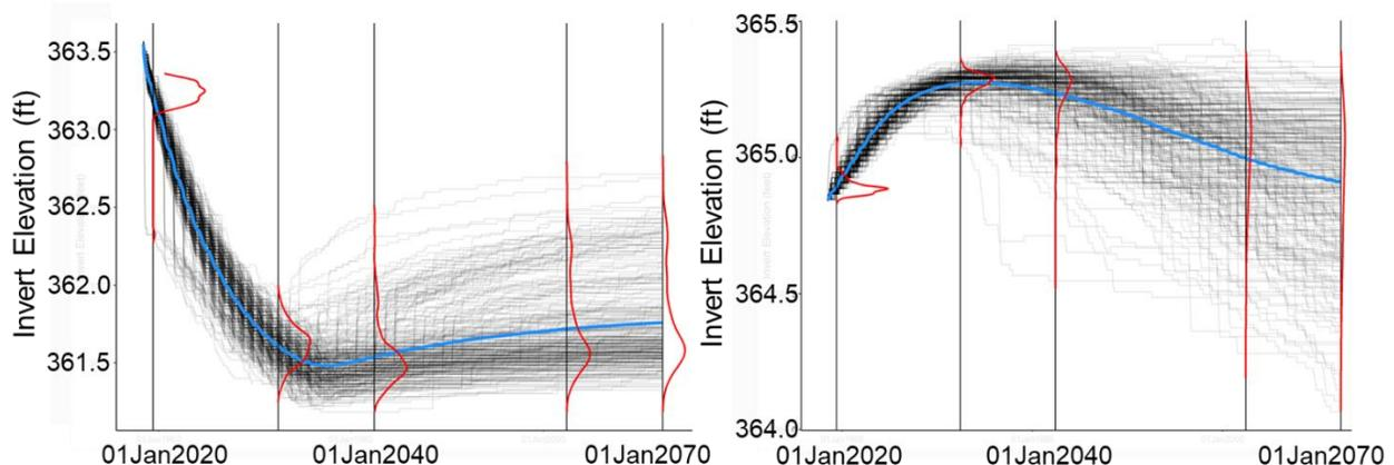
**Figure 3.** HEC-RAS bed change time series traces at two cross section on the Missouri River. Plots include 350 realizations based on stochastic 50-year future hydrologies provided by HEC-WAT. Blue line is mean and red lines are proportional distributions.
