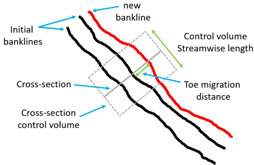
**Figure 5.** Schematic of bank planform area change computation.
