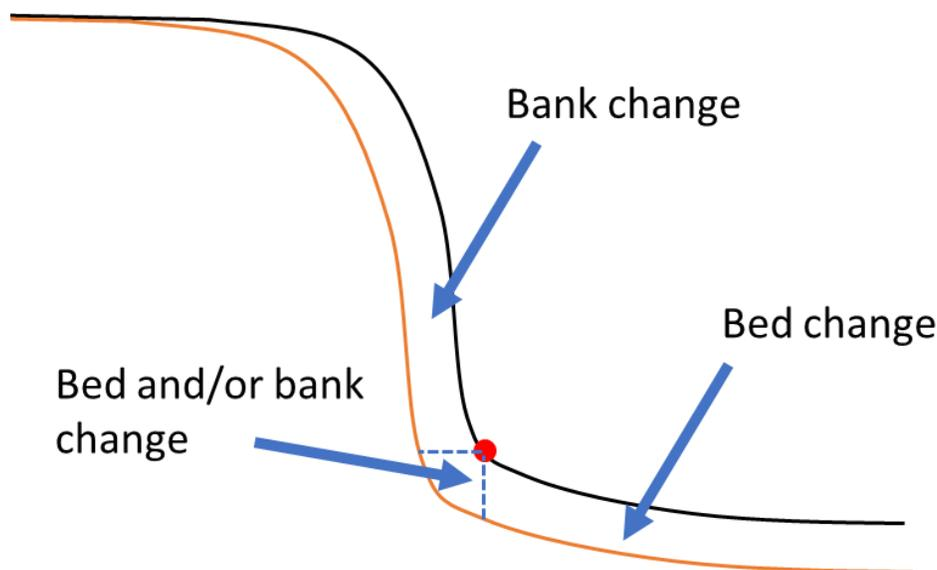
**Figure 4.** A schematic of cross-section change as computed from survey data. Cross section change in the vicinity of the bank toe can be attributed to bed change, bank change, or some combination of the two.
